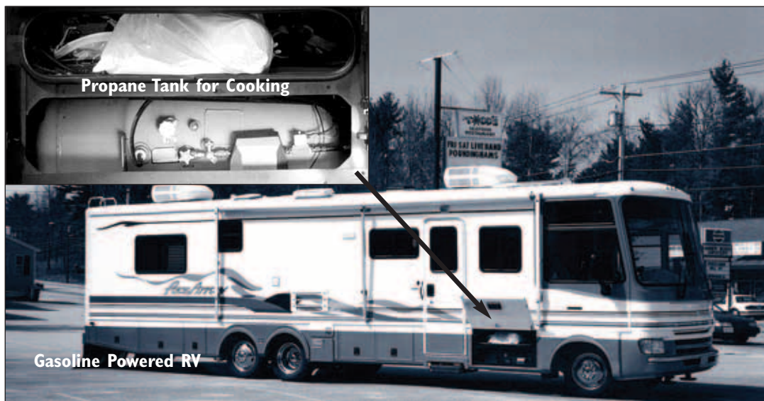
FIGURE 4-16 Mobile RV tanks should not be confused with the vehicles fuel tank.
