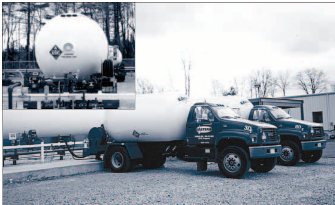
FIGURE 6-11 Bobtail loading station.
