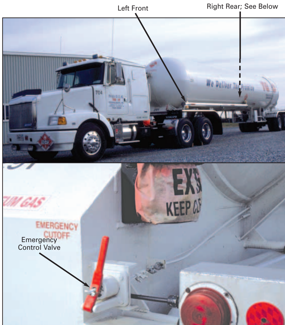
FIGURE 5-8 Location of Emergency Controls on MC-331
