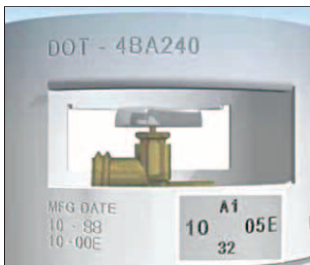
FIGURE 4-13 Cylinder with RIN (A132) and external inspection date (10-05).
