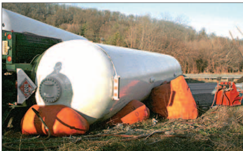
FIGURE 9-19 Air bags are usually not effective for uprighting bobtails and MC-330/331 containers.
