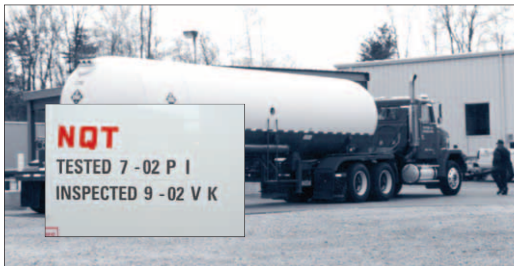
FIGURE 5-15 Cargo tank inspection markings.
