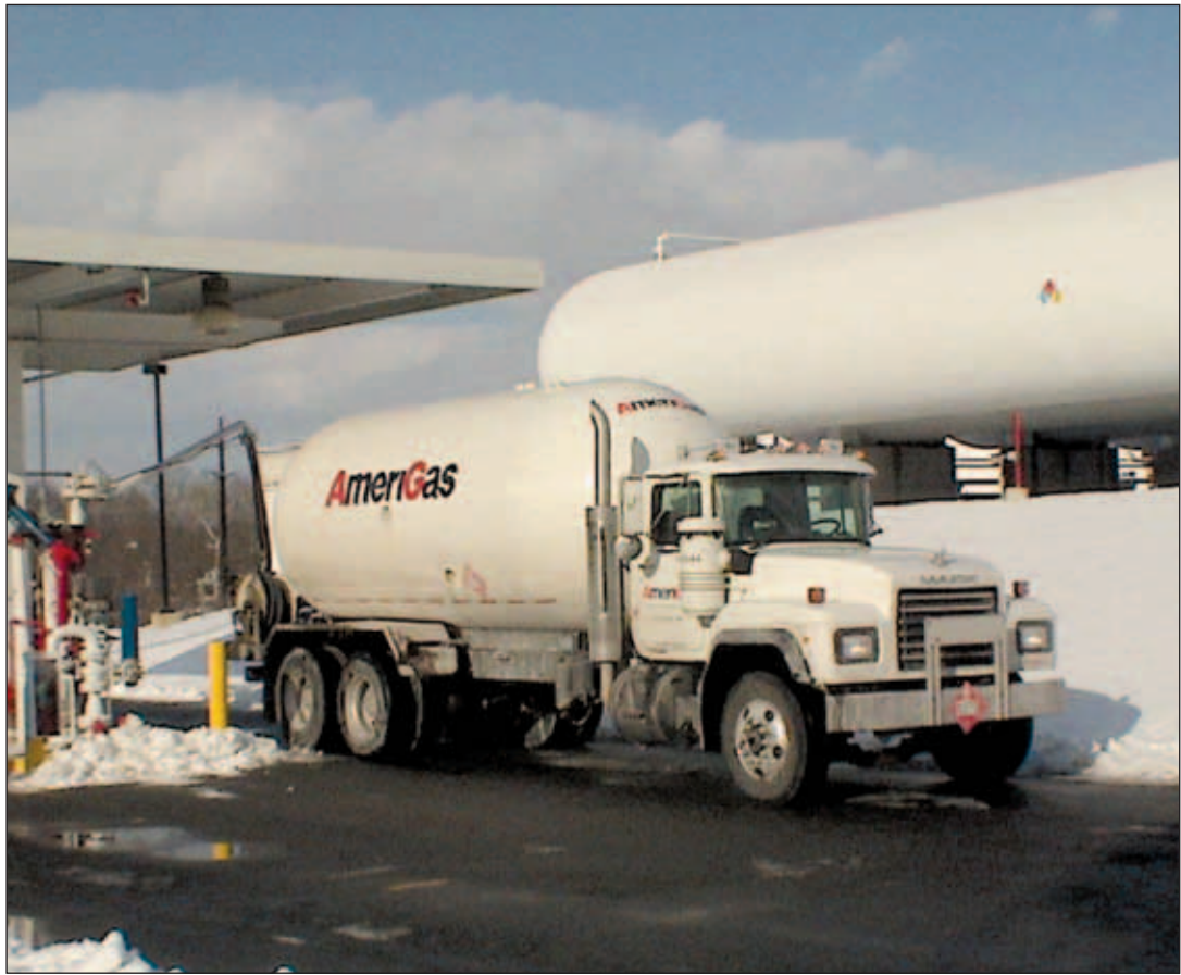
FIGURE 6-1 MC-331 bobtail cargo tank truck being filled at a bulk plant.
