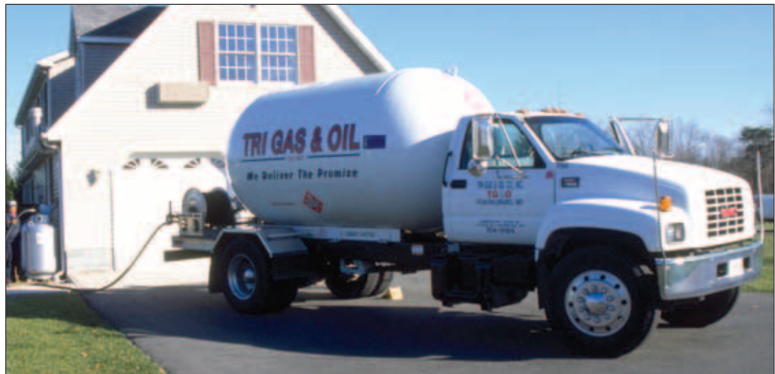
FIGURE 6-10 The bobtail truck is the primary method of delivering propane to customers.
