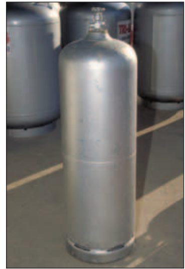
FIGURE 4-8 DOT portable exchange cylinder. These cylinders are filled by a propane dealer and transported to the customer's site.
