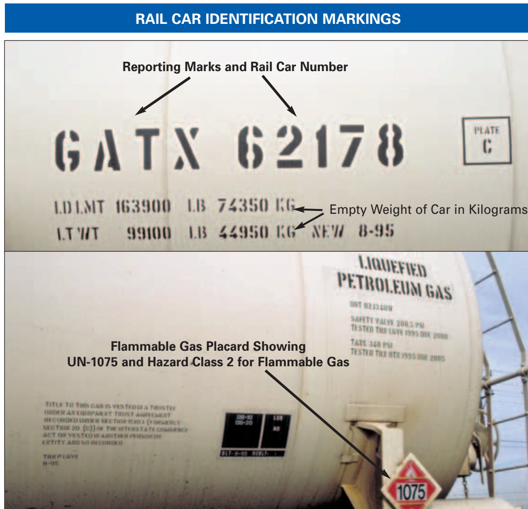
FIGURE 5-17 Railroad tank car identification markings.
