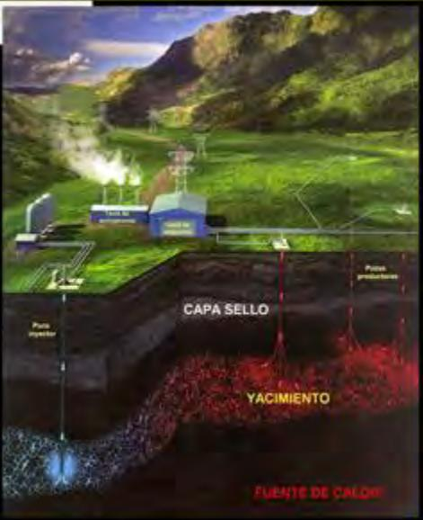
Diagram illustrating the conceptual model of a geothermal reservoir. It shows a well labeled "Pozo inyector" (Injection Well) on the left, a "CAPA SELLO" (Sealing Layer) in the middle, a "YACIMIENTO" (Reservoir) containing a "FUENTE DE CALOR" (Heat Source) at the bottom, and a "Pozo productivo" (Production Well) on the right.
