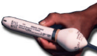
Satellite pop-off tag.—this instrument records temperature, depth and light levels while attached to the whale shark.
