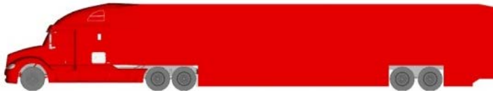
Gap Seal + Skirt + 32" Boattail (3-sided)
