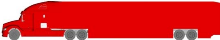
Gap Seal + Skirt + 32" Boattail (4-sided, hi)
