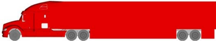
Gap Seal + Skirt + 24" Boattail (3-sided)
