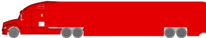
Gap Seal + Skirt + 32" Boattail (3-sided)
